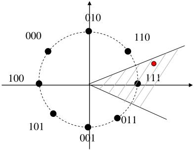
In 8PSK modulator, every 3 bits are mapped to one complex-valued 8PSK symbol. The transmitted symbols are corrupted by both Rayleigh flat fading and additive white Gaussian noise.
