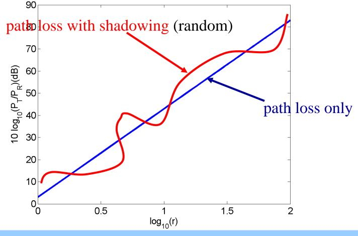
combined effects of path loss and shadowing (red curve)
