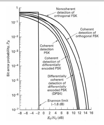
Coherent detection PSK > coherent detection of differentially encoded PSK > Differential detection of differentially encoded PSK (DPSK) > Coherent detection of orthogonal FSK > Noncoherent detection of orthogonal FSK.
