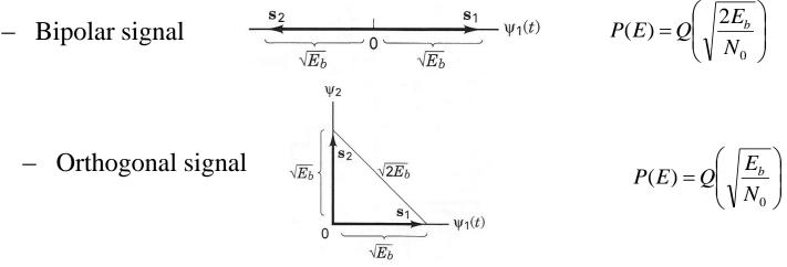
•  $E_d$  is the squared distance between the two modulation points.
