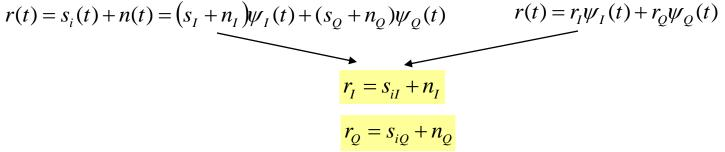
The bandpass communication system is equivalently represented as the summation of signal vector and noise vector
