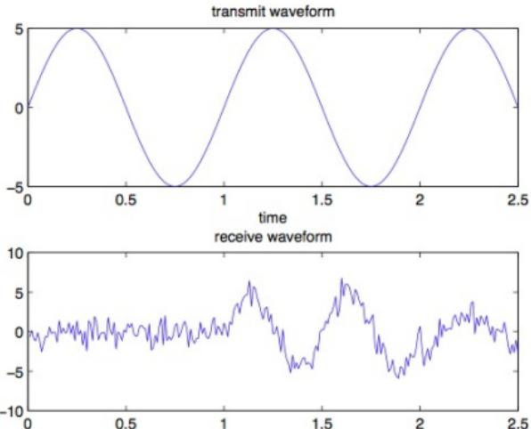
The received waveform is time-dilated and shifted version of original waveform  $g(t)$  plus noise
