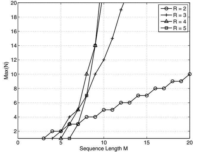
Fig. 2. Maximum number of users supported by a CT-MAC system with the OOAT. ( $N$ : number of users;  $M$ : number of sub-symbols/symbol;  $R$ : number of repetitions per symbol.)
