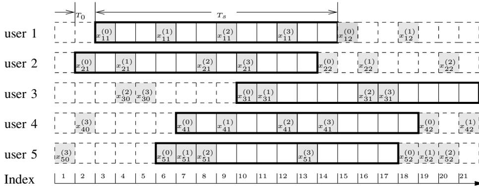
Fig. 1. An OOAT system with  $N = 5$  users,  $R = 4$  repetitions per symbol period, and each symbol contains  $M = 12$  possible sub-symbol positions.
