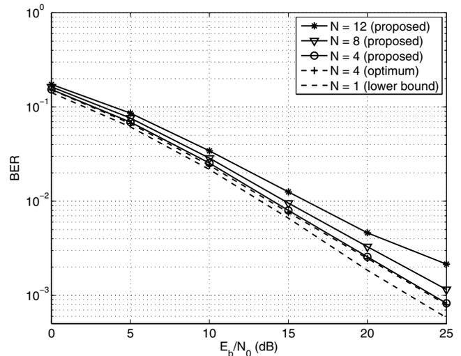
Fig. 3. BER performance of a system with  $M = 12$  sub-symbols/symbol,  $R = 4$  repetitions, and the sub-optimum iterative detection method.
