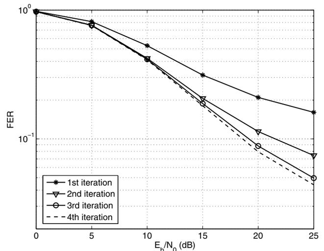
Fig. 4. FER performance of a system with  $M = 12$  sub-symbols/symbol,  $R = 4$  repetitions,  $N = 12$  users, and the sub-optimum detection method.
