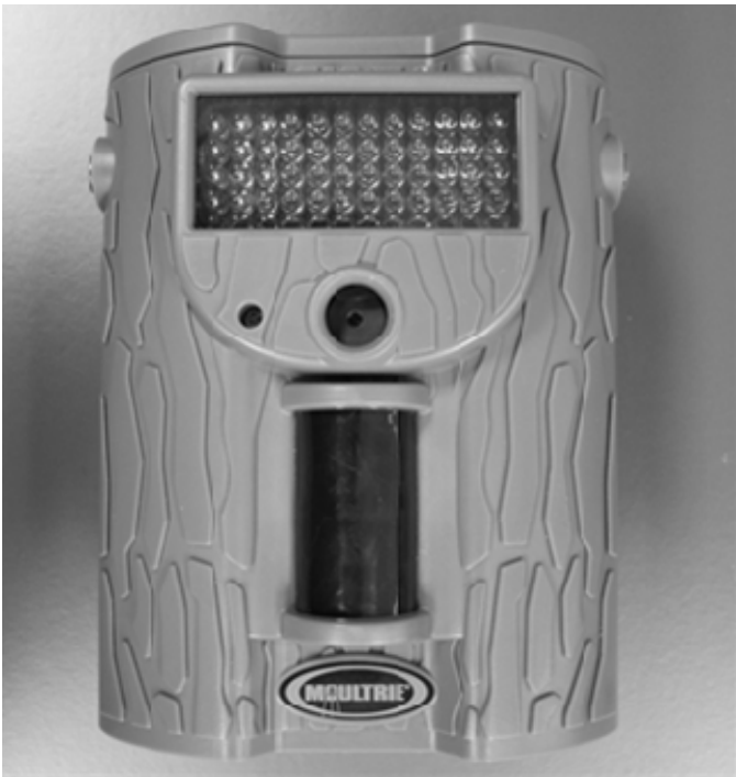
Figure 1: Camera in Weatherproof Enclosure
