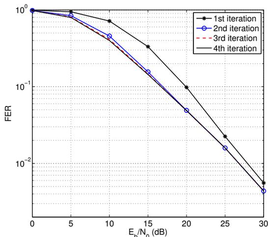
Fig. 4. FER performance of the system with  $M = 10$  slots,  $N = 20$  users,  $R = 2$  repetitions, and the message passing algorithm.
