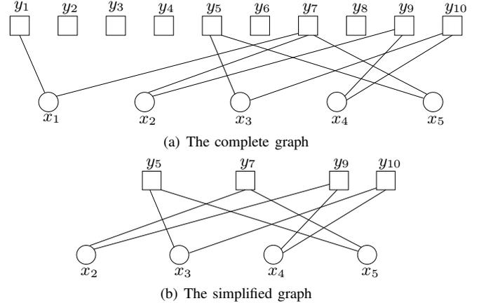
Fig. 1. Graph representations of a CT-MAC system with  $N = 5$  users,  $M = 10$  slots, and  $R = 2$  repetitions.
