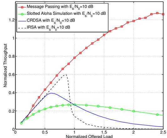
Fig. 5. Normalized throughput v.s. normalized offered load.
