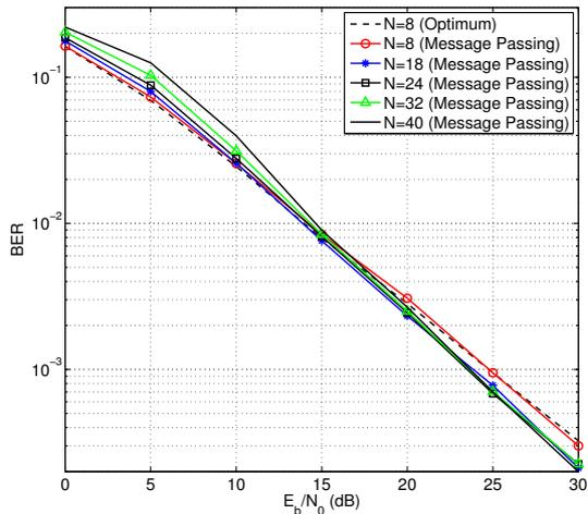
Fig. 3. BER performance of the system with  $M = 12$  slots,  $R = 2$  repetitions, and the message passing algorithm.
