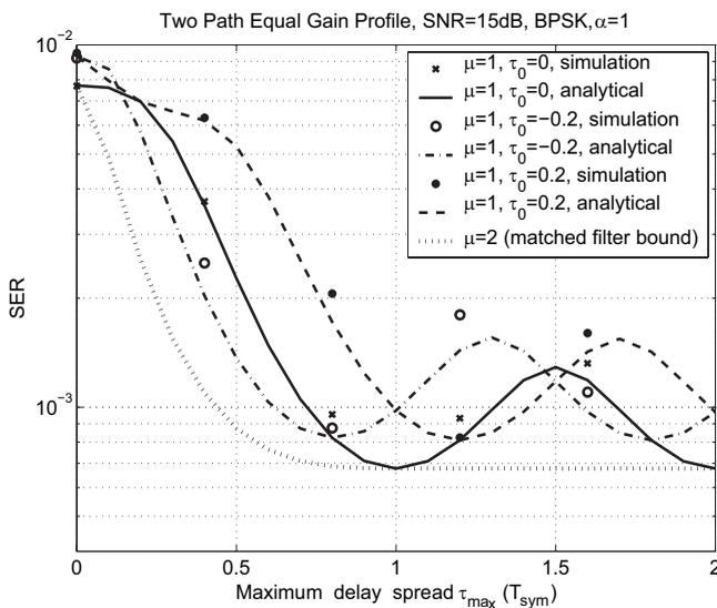
Fig. 7. The SER performance of systems with two-path equal gain profile with respect to the maximum delay spread of the channel (or the relative delay between the two channel paths).  $\mu$ : oversampling factor.  $\tau_0$ : receiver timing phase offset.  $\alpha = 1$ : roll-off factor of the RRC filter.
