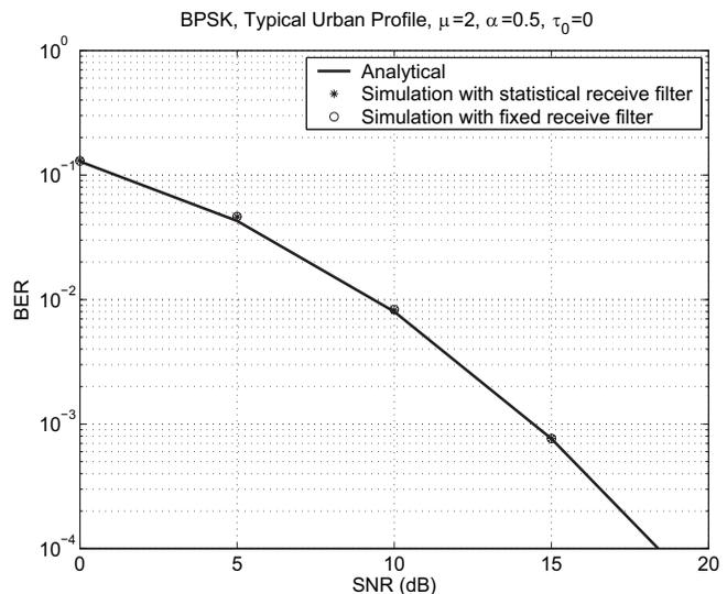
Fig. 3. Comparison of the performance of ISI-removed systems with fixed receive filter and statistical receive filter.  $\mu = 2$ : oversampling factor.  $\tau_0 = 0$ : receiver timing phase offset.  $\alpha = 0.5$ : roll-off factor of the RRC filter.
