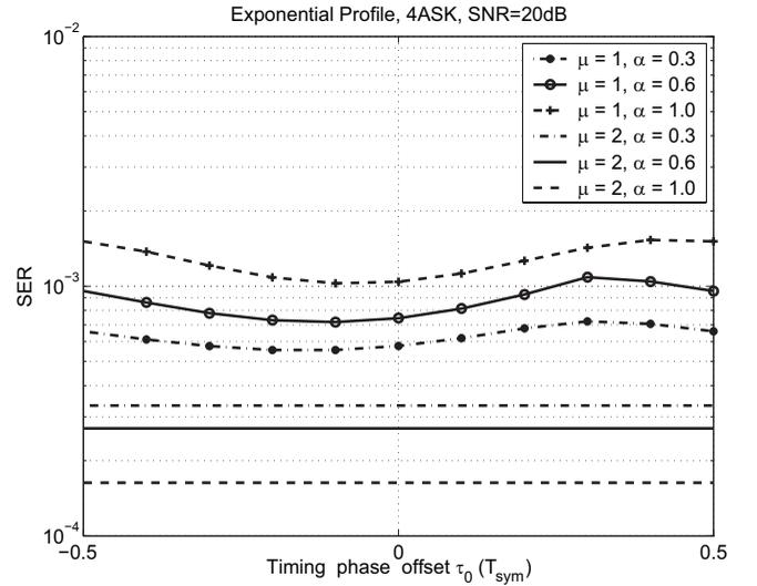
Fig. 6. The effects of receiver timing phase and excessive bandwidth on the error performance of system with Exponentially Decaying profile with  $\tau_{max} = 3T_{sym}$ .  $\mu$ : oversampling factor.  $\alpha$ : roll-off factor of the RRC filter.
