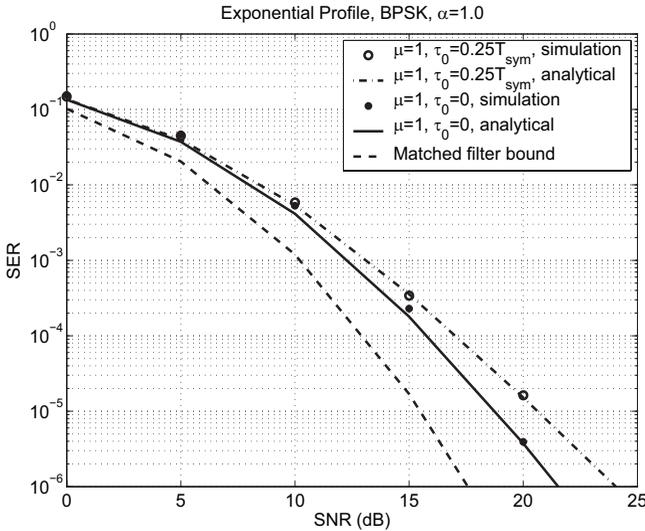
Fig. 5. Comparison of performance bounds with simulation results of systems with Exponentially decaying profile. Block length for the MAP equalizers: 1024 symbols.  $\mu$ : oversampling factor.  $\tau_0$ : receiver timing phase offset.  $\alpha = 1$ : roll-off factor of the RRC filter.
