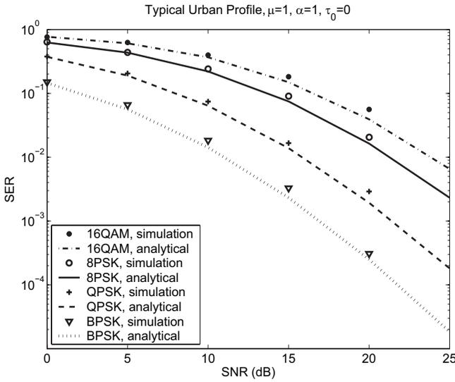
Fig. 4. Comparison of performance bounds with simulation results of systems with Typical Urban profile and various modulation schemes. Block length for the MAP equalizers: 256 symbols.  $\mu = 1$ : oversampling factor.  $\tau_0 = 0$ : receiver timing phase offset.  $\alpha = 1$ : roll-off factor of the RRC filter.
